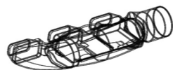
Fig. 1. 3-D geometry of the flow section of the intake manifolds of the standard design
