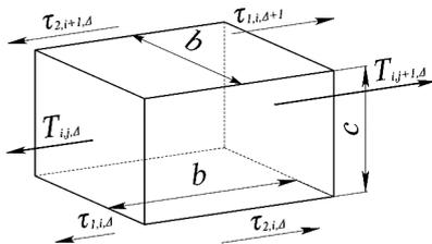
Fig. 1. Arbitrary abrasive grain loaded with a force directed along the  $j$  axis parallel to the working plane
