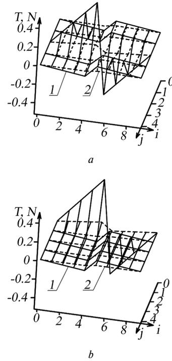
Fig. 2. Distribution of forces between the abrasive grains in the working layer (Curve 1) and the layer under it (Curve 2) when loading the middle (a) and extreme (b) grains in the middle row
