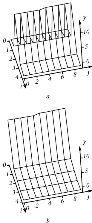
Fig. 4. Tangents of mutual shear angles of abrasive grains in the working layer when loading the middle:
