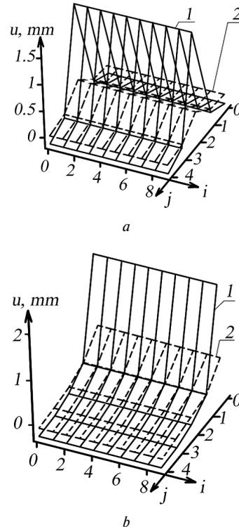
Fig. 3. Displacement of abrasive grains in the working layer (Curve 1) and the layer under it (Curve 2) when loading the middle (a) and extreme (b) grains in the middle row
