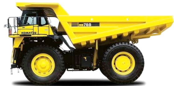
Fig. 5. KOMATSU HD785-7 mining auto-train [22]
