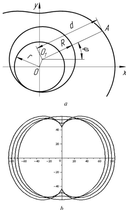
Fig. 3. Diagram of forming the working profile of the body of the RPM:
