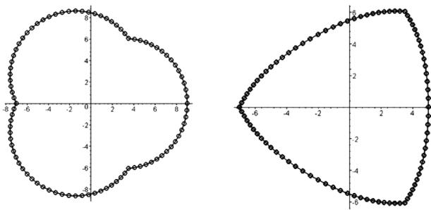
Fig. 5. Contours of the rotor working surfaces and the body of the RPM
