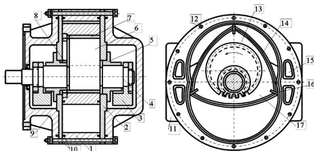
Fig. 1. Design variant of the RPM with an epitrochoid contour of the working cavity ( $m = 3/2$ )
