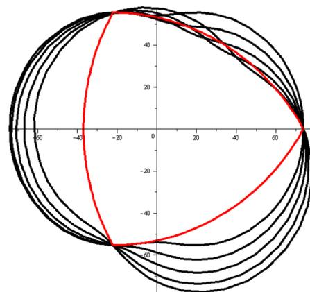
Fig. 4. Diagram of movement of the epitrochoid relative to rotor profile
