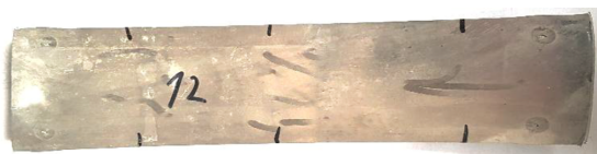
Fig. 3. View of the composite after rolling
