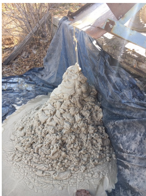
Fig. 5. The stockpile of deslamed marketable sand
