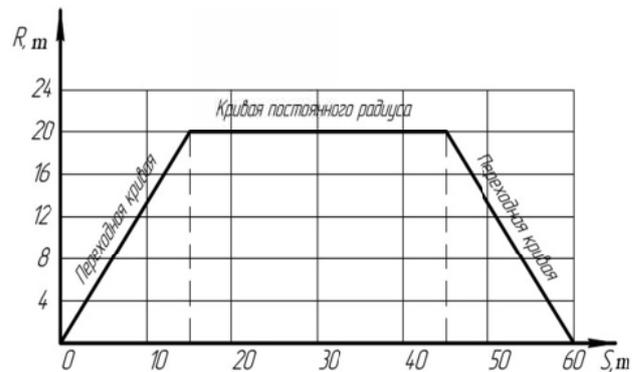
Fig. 3. Macrogeometry of rail track in horizontal surface:  $R$  – bending radius, m
