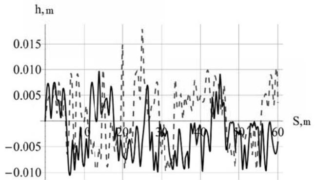
Fig. 2. Vertical trajectory of wheel center displacement:  $h$  – height of rail track irregularities, m;  $S$  – track length, m; ——— irregularities of the left rail; - - - - irregularities of the right rail
