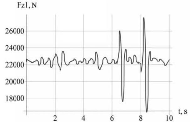
Fig. 1. The value of reactive loading, which takes wagon's wheel (of the left rail):  $F_{z1}$  – rail reaction under oncoming wheel, N;  $t$  – simulation time, s
