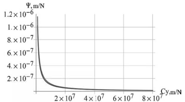
Fig. 8. Relation of output member axle flexibility to EDE rigidity:  $\psi$  – EDE flexibility, m/N
