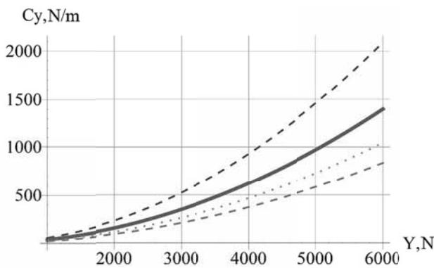
Fig. 6. Relation of EDE axle rigidity to guiding force:  $C_y$  – EDE axle rigidity, N/m;  $Y$  – value of guiding force, N
