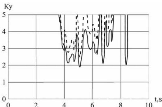
Fig. 9. Relation of momentary SC value to track features:  $K_y$  – safety coefficient: ——— fixed mounting of oncoming wheel; - - - - - movable mounting of oncoming wheel with EDE
