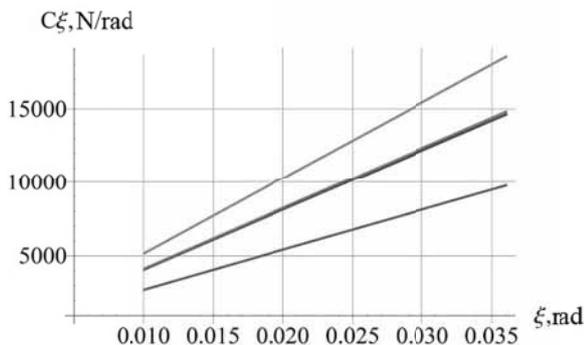
Fig. 7. Relation EDE angular rigidity to angular displacement:  $C_\xi$  – EDE angular rigidity, N/rad;  $\xi$  – value of output member angular displacement, rad
